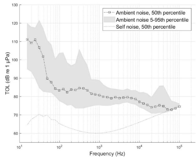
Fig. 3. Third octave levels of deep-water ambient noise from the deepest channel (~695 m) of one deep water deployment lasting 5 h. TOLs were calculated over 30 s intervals. The self noise of the SoundTrap is also shown, illustrating that ambient noise measurements were limited by self noise above about 30 kHz in this location.
