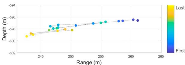
Fig. 2. Range-depth track constructed from localised clicks ( $n = 20$ ) in a pilot whale click train over a 12 s period, demonstrating that the array can be used to track the diving behaviour of deep-diving toothed whales. Range shown is relative to the central channel on the array.
