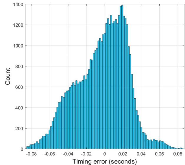
Fig. 4. Time synchronisation errors for six SoundTraps on the array with respect to the seventh recorder which acted as the timing master. This distribution was taken from one field deployment ( $n = \sim 43,800$  acoustic timing pings) recording at a sample rate of 576 kHz.
